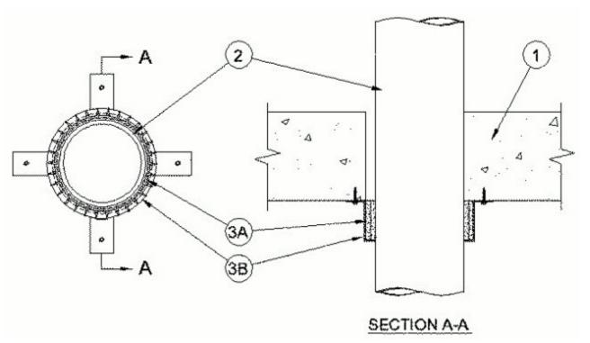
1. **Floor or Wall Assembly** — Min 4-1/2 in. (114 mm) thick reinforced lightweight or normal weight (100-150 pcf or 1600-2400 kg/m³) concrete. Wall may also be constructed of any UL Classified **Concrete Blocks\***. The diam of opening shall be 5 in.(127 mm)
