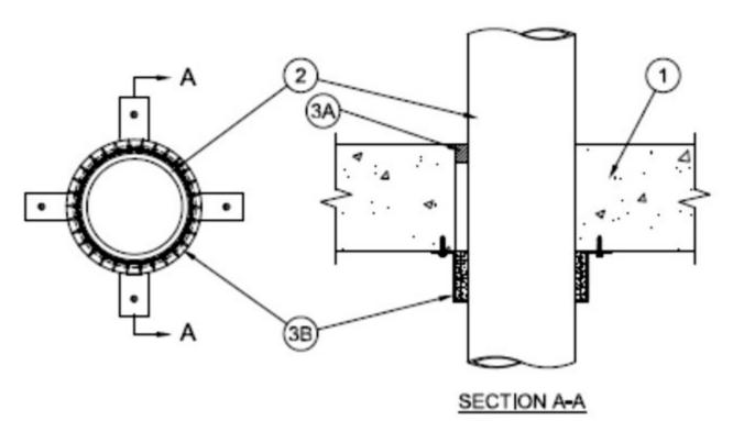
1. **Floor or Wall Assembly** — Min 4-1/2 in. (114 mm)thick reinforced lightweight or normal weight (100-150 pcf 1600-2400 kg/m³) concrete. Wall may also be constructed of any UL Classified **Concrete Blocks\***. Floor may also be constructed of any min 6 in. (152 mm) thick UL Classified hollow-core **Precast Concrete Units\***. Max diam of opening is 5 in. (127 mm).
