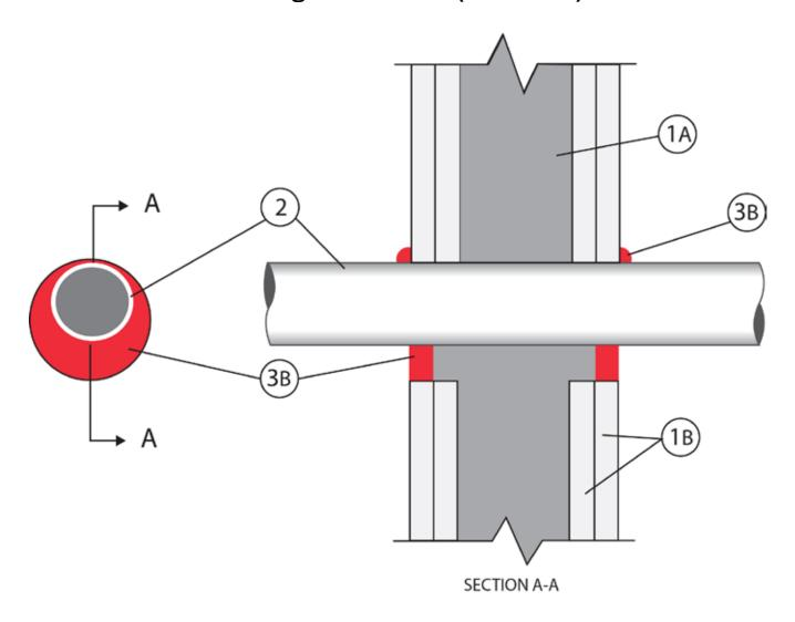
1. Wall Assembly — The 1 or 2 hour fire-rated gypsum board/stud wall assembly shall be constructed of the materials and in the manner specified in the individual U300 or U400 Series Wall and Partition Designs in the UL Fire Resistance Directory and shall include the following construction features:
